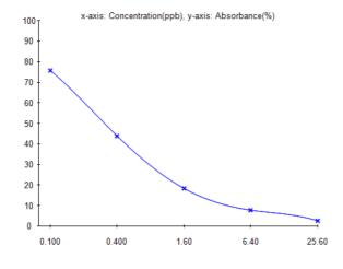
Spline Standards Conc.(ppb) / A(Mean) 0.100 1.633 (Coeff. of Var.: 1.7%) 0.400 0.946 (Coeff. of Var.: 0.5%) 1.60 0.396 (Coeff. of Var.: 2.1%) 6.40 (Coeff. of Var.: 0.0%) 25 60 0.057 (Coeff. of Var.: 5.0%) 50% inhibition: 0.309
