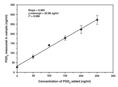
Measurement of PGD2 in cell lysates. Cells were lysed as described in the Sample Preparation section. The lysates were then spiked with PGD2, diluted with ELISA Buffer, and analyzed using the PGD2 ELISA Kit. The y-intercept corresponds to the amount of PGD2 measured in unspiked lysates. Error bars represent standard deviations obtained from multiple dilutions of each sample.
