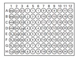
Blk - Blank TA - Total Activity NSB - Non-Specific Binding B<sub>0</sub> - Maximum Binding S1-S8 - Standards 1-8 1-24 - Samples
