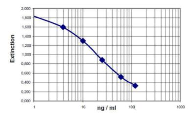
If the extinction of a sample lies below the value of calibrator 6 (120 ng/ml), the result should be given as ">120 ng/ml". It is recommended that the sample be re-tested at a dilution of 1:2 with calibrator 1 before following the test instructions. The result in ng/ml read from the calibration curve for this sample must then be multiplied by a factor of 2.
