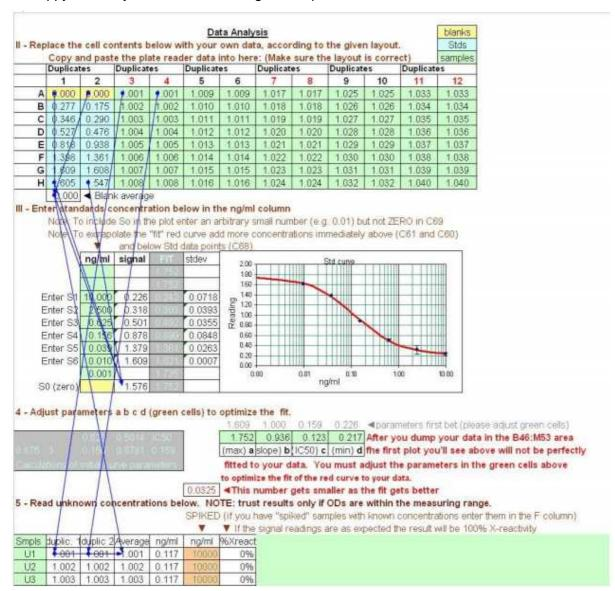
Set up an 8 x 12 area to match the layout of the plate and copy the plate reader data in it. Calculate the average of the blanks on another cell as indicated by the arrows starting from cells A1 and A2.
