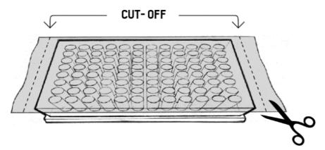
Note: This is to ensure the temperature distribution is evenly spread out in all wells from bottom and sides; any extra parafilm can be cut off once the top is sealed to block evaporation.
