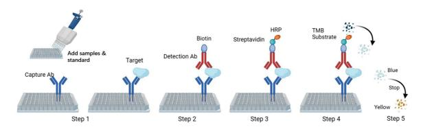
Step1: Add 100 µl standard or sample to each well and incubate for 90 minutes at 37°C.
