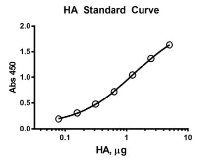
A sample titration using human serum with a 2 hour reaction time. Data interpolated against an HA standard curve and analyzed using non-linear regression analysis with GraphPad Software.
