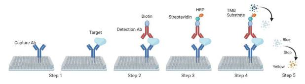
Step1: Add 100 µL standard or sample to each well and incubate for 90 minutes at 37°C.
